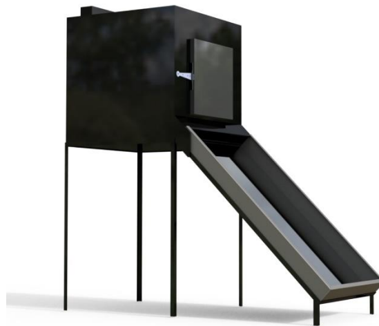
Figure 16: Solar drying system to transform Transforming protein Hydrolysate solution to solid form
