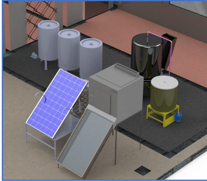
Figure 7 : Glue production system with Solar Heating and Biomass backup heater and solar glue drier
