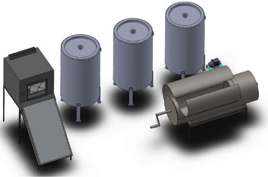
Figure 26 : Overall salt recovery system with solar drying system to produce solid salt
