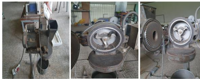
Figure 17: Small-scale motorized grinding machine to change solid material to powder form (Chemical Engineering Laboratory, Addis Ababa Institute of technology)
