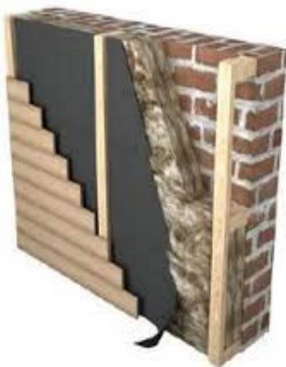
Figure 4.6-7 - Scheme of ventilated facade composition on a brick wall with wooden bearing structure
