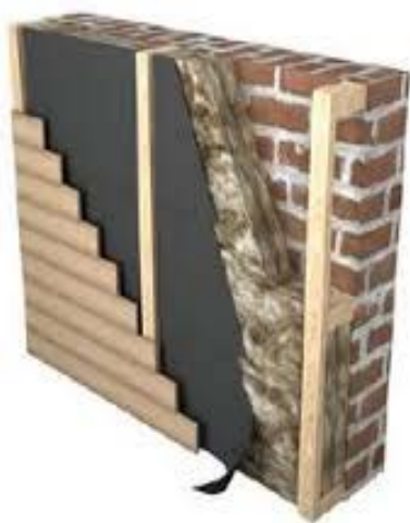
Figure 4.6-1 - Scheme of ventilated facade composition on a brick wall with wooden bearing structure
